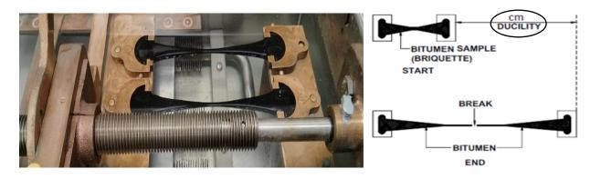
Figure 14.4: Ductility Testing
