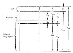
Figure 1.2Representation of volumes in a compacted asphalt specimen
