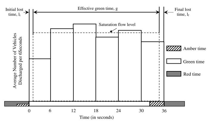
**Figure 8.1** A typical example for fixed-time signals showing the variation of average discharge rate during a fully saturated green period
