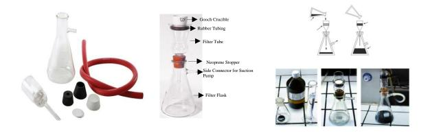
Figure 13.1: Component parts of the filtering apparatus
