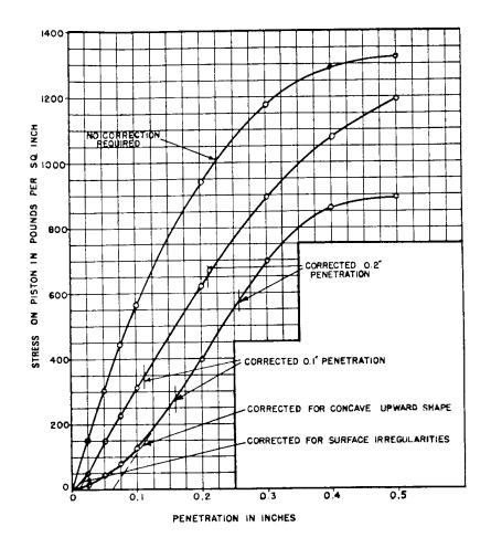
*NOTE: See Table 2 for metric equivalents* **Figure 16.2:** Correction of Load-Penetration Curves
