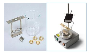
Figure 12.1 Ring and Ball apparatus
