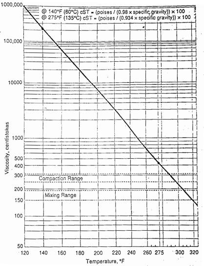
Figure 17.4 Determination of Mixing and Compaction Temperatures
