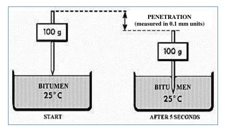
Figure 11.2: Penetration test
