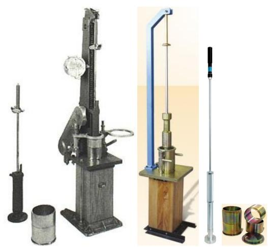
Mechanical compaction hammer assembly
