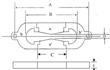
Figure 14.1 Mold for Ductility Test Specimen
