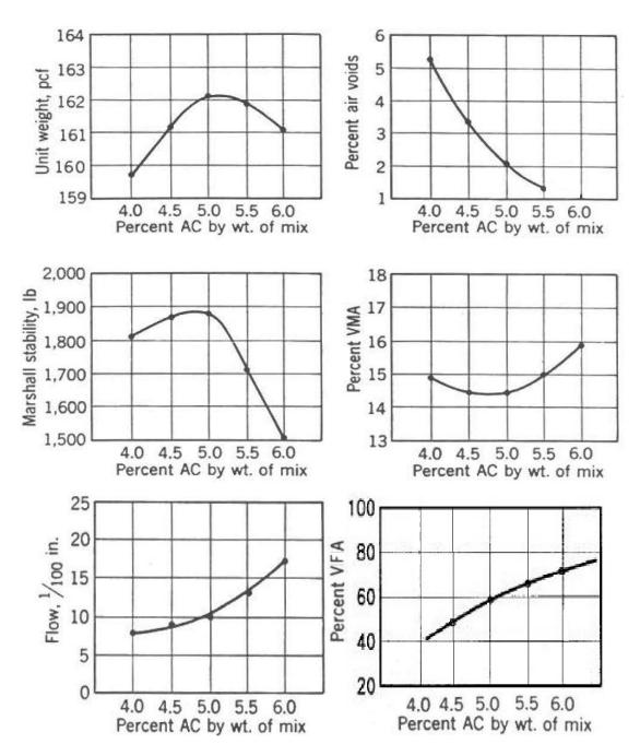
**Figure 17.6** Test property curves for hot-mix design data by the Marshall method (Reference book: "Highway Materials" by Robert D. Kerbs& Richard D. Walker. Figure 12.3, Page-398)
