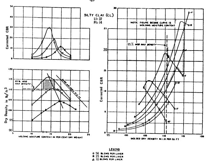
NOTE Surcharge = 50 lb soaking and penetration. All samples soaked top and bottom four days. All samples compacted in 5 layers, 10-lb hammer, 18-in. drop in CBR mold.
