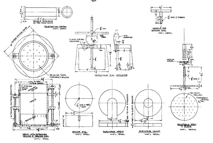
Figure 16.1: Bearing Ratio Test Apparatus (See Table 16.2 for metric equivalents)
