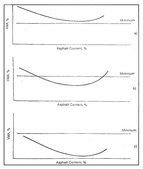
Figure 17.8 Relationship between VMA and specification limit
