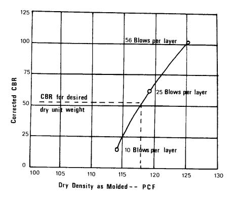
Figure 16.3 Dry Density Versus CBR
