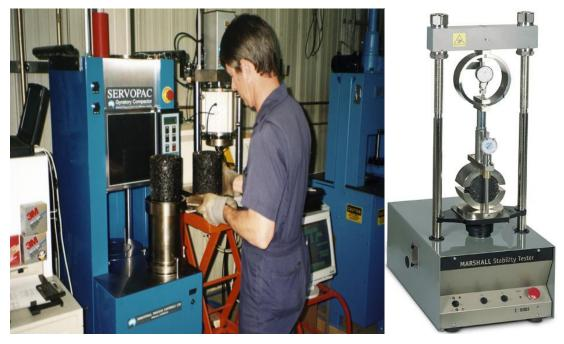
Figure 17.5 Marshall stability and flow test
