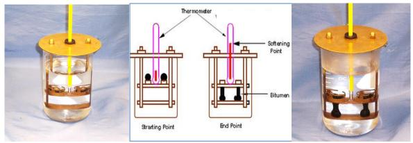
Figure 12.2 Illustration of softening point
